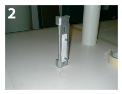
Place punched plastic spacer over stove bolt on face and slide all the way down. Place second stove bolt from behind through elongated hole and through plastic spacer as shown.
